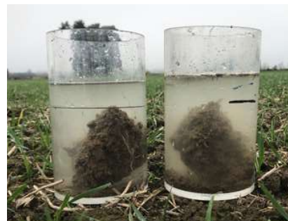
Figure 4. Samples showing the difference between a high and low turbidity score.
