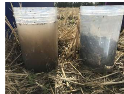
Figure 4. Samples showing the difference between a high and low turbidity score.
